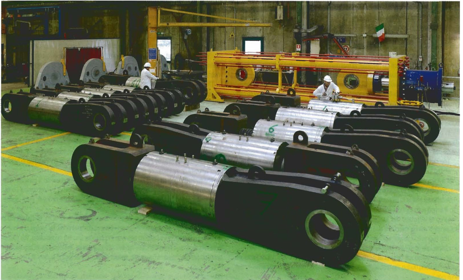
Ten shock transmission units awaiting painting at the factory. The testing equipment is shown in the background
