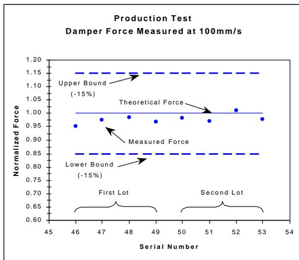
Figure 11 - Normalized reaction of the production units.
