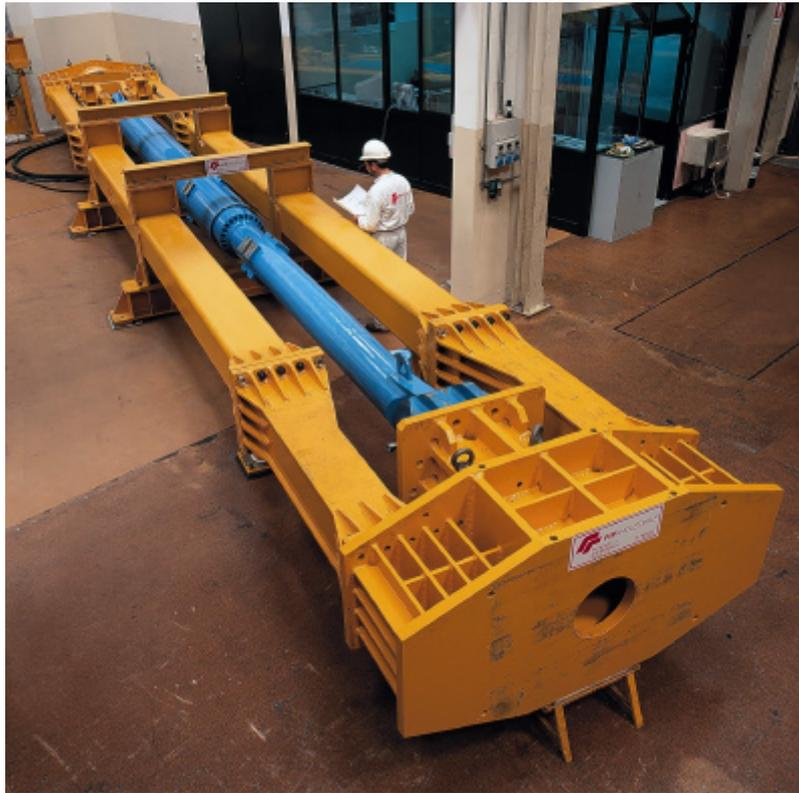
Figure 10 - Production tests at FIP laboratory on a fluid viscous damper for the main bridge.
