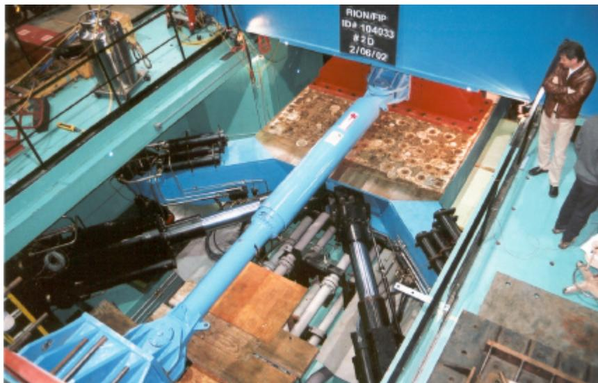
**Figure 7 - Prototype testing at SRMD Facility (UCSD).**
