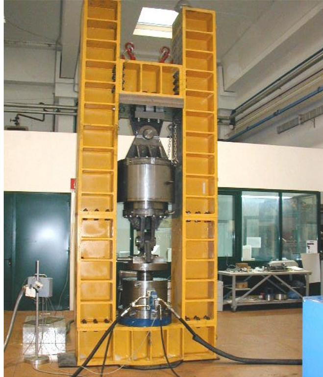
**Figure 16 - SR1050 Fuse element during fatigue test.**
