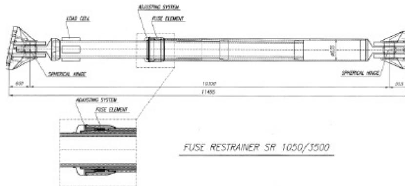
**Figure 3 - General configuration of fuse restraint installed on main pylons.**
