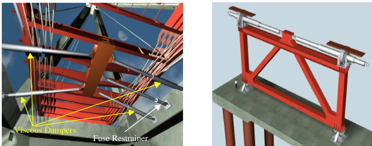
**Figure 2 - Rion Antirion Main Bridge: arrangement of fluid viscous dampers on the main piers (left) and on the transition piers (right).**
