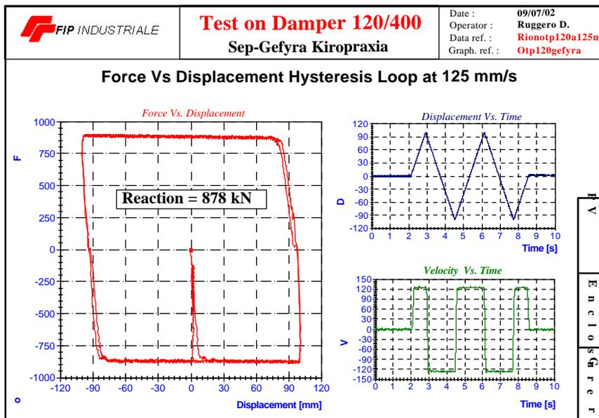
**Figure 14 - Hysteresis Loop measured in a constant velocity test .**
