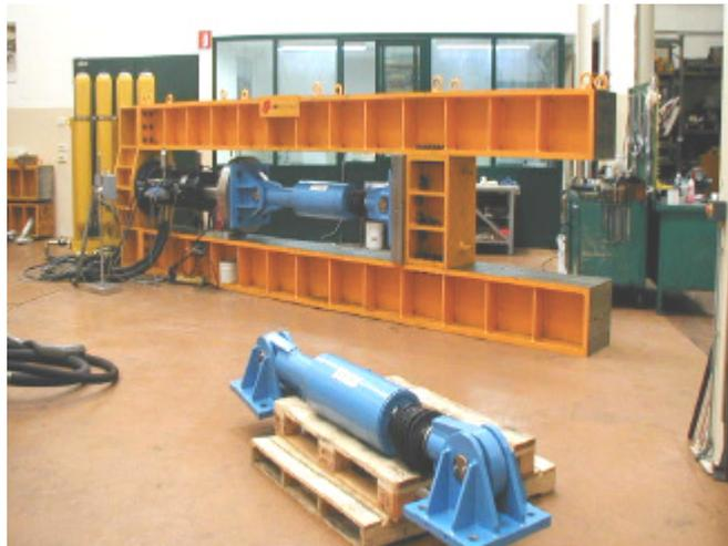
**Figure 13 - Production Tests at FIP Laboratory on a longitudinal damper for the Antirion Approach Viaduct.**
