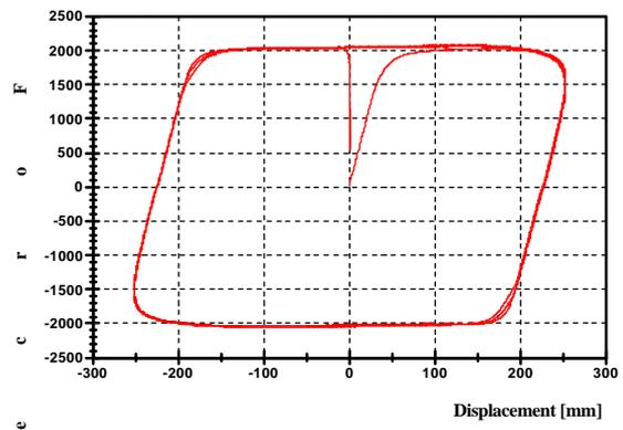
Figure 12 – Hysteresis loop measured in sinusoidal dynamic tests at  $V_{max}=175$  mm/s on a transition pier damper.
