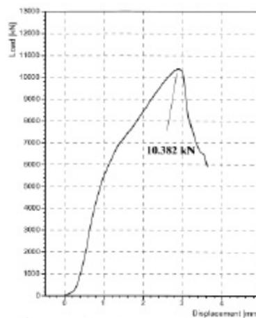
**Figure 15 - Failure test results on Fuse Restraints SR340 (left) and SR1050 (right).**
